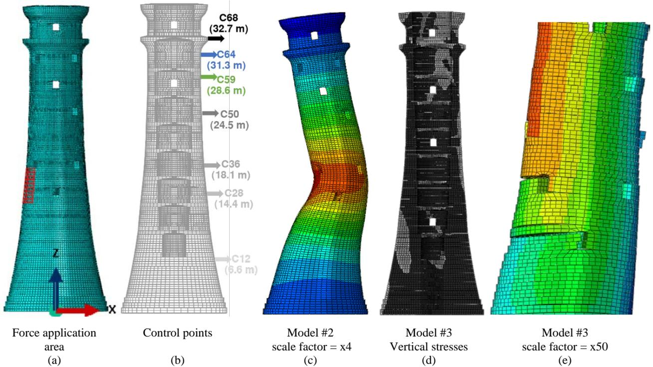
Figure 5. FE model of Fastnet lighthouse: (a) red lines indicating area of application of impulsive forces; (b) control points; (c) homogeneous nonlinear model deformed shape (scaled exaggerated); (d) vertical stresses for interface model; (e) joint opening for interface model (scaled exaggerated)
