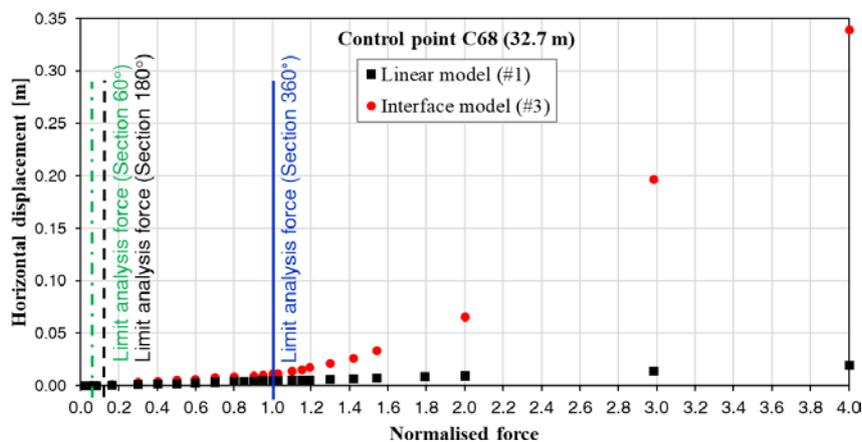
Figure 7. Horizontal displacement at control point C68 at 32.7m for the FE models #1 and #3 together with threshold levels of forces calculated based on the limit analysis method
