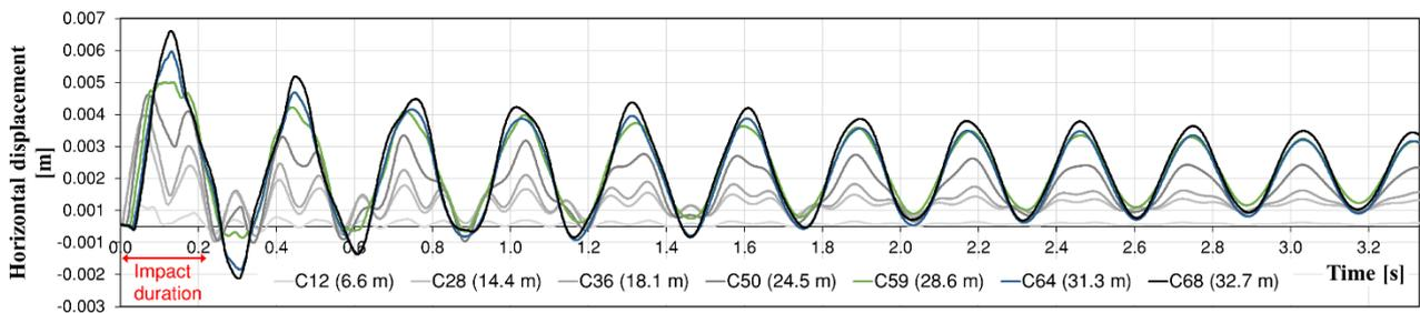
Figure 6. Structural response of model #3 for the generic wave with impact area between 13.0 m and 17.1 m: horizontal displacements recorded at the control points
