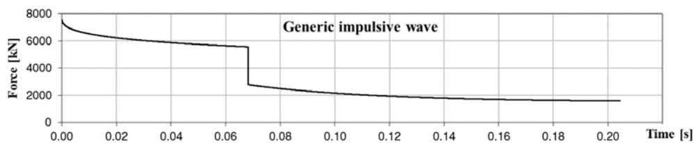
Figure 4. Time-history of the impulsive wave total force applied on the structure
