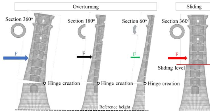
Figure 2. Failure mechanism for limit analysis: (a) overturning for  $360^\circ$  section, (b) overturning for  $180^\circ$  section, (c) overturning for  $60^\circ$  section, (d) sliding for  $360^\circ$  section
