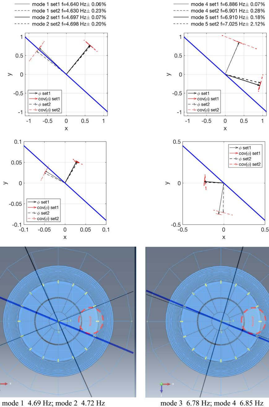
**Fig. 10.** Wolf Rock first (left columns) and second (right columns) mode pairs. Level 9 (upper) and 8 (middle). FEM modes (lower), red curve locates upper door. (Thick) blue lines are in direction of landing platform (also the entrance). (For interpretation of the references to colour in this figure legend, the reader is referred to the web version of this article.)
