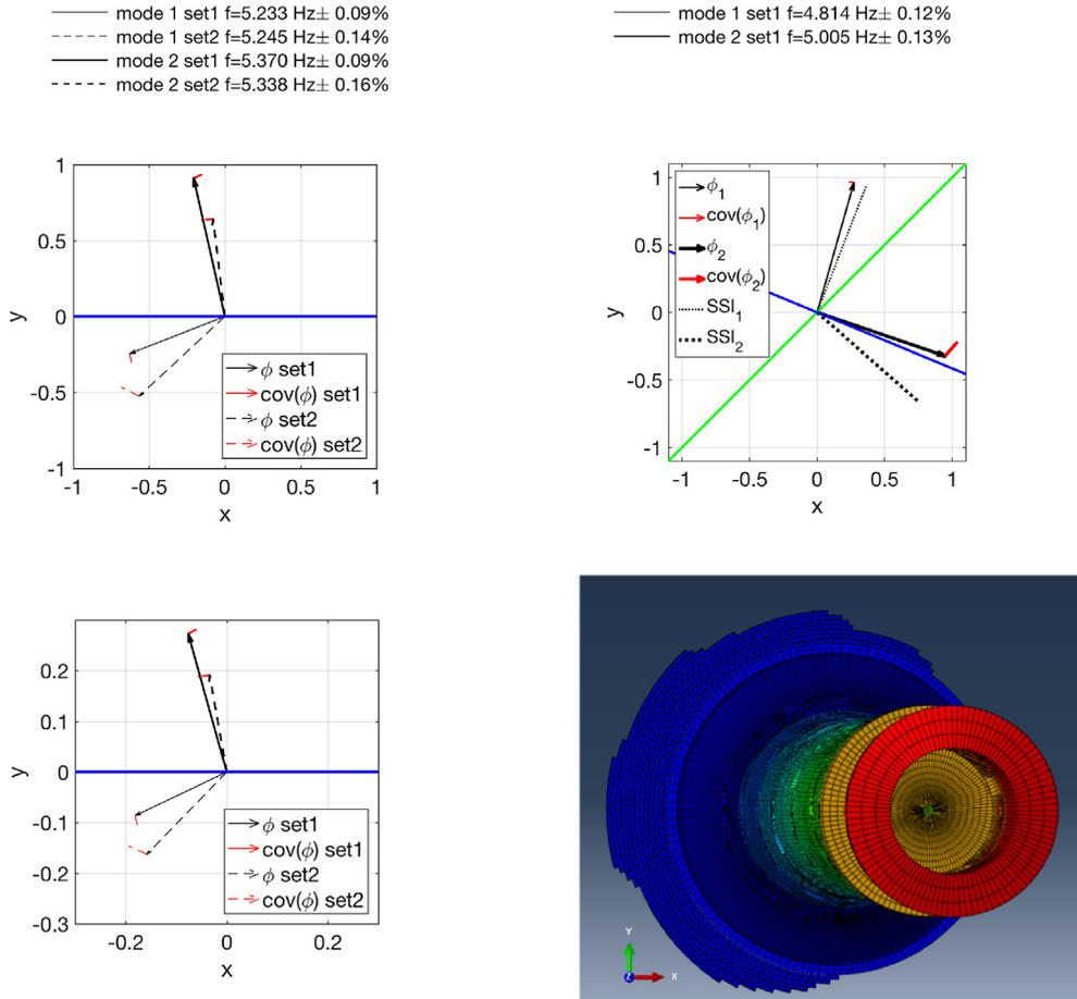
**Fig. 11.** Left column Dubh Artach level 7 (upper) and level 3 (lower); x axis (blue line) is aligned with openings (windows, doors). Right column Fastnet; x axis aligns with entrance, green line is North-South axis, blue line is x axis of FEM. FEM second mode, along the model axes shown bottom right. (For interpretation of the references to colour in this figure legend, the reader is referred to the web version of this article.)
