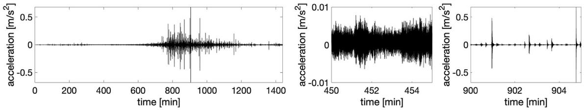
**Fig. 13.** Wolf Rock acceleration response during ex-Hurricane Ophelia, 16th October 2017. Left, for the whole day, middle for 7.30 AM (low tide), right for 3 PM.
